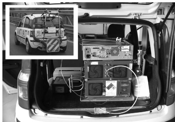
Fig. 5. Passenger car instrumented with PEMS.
